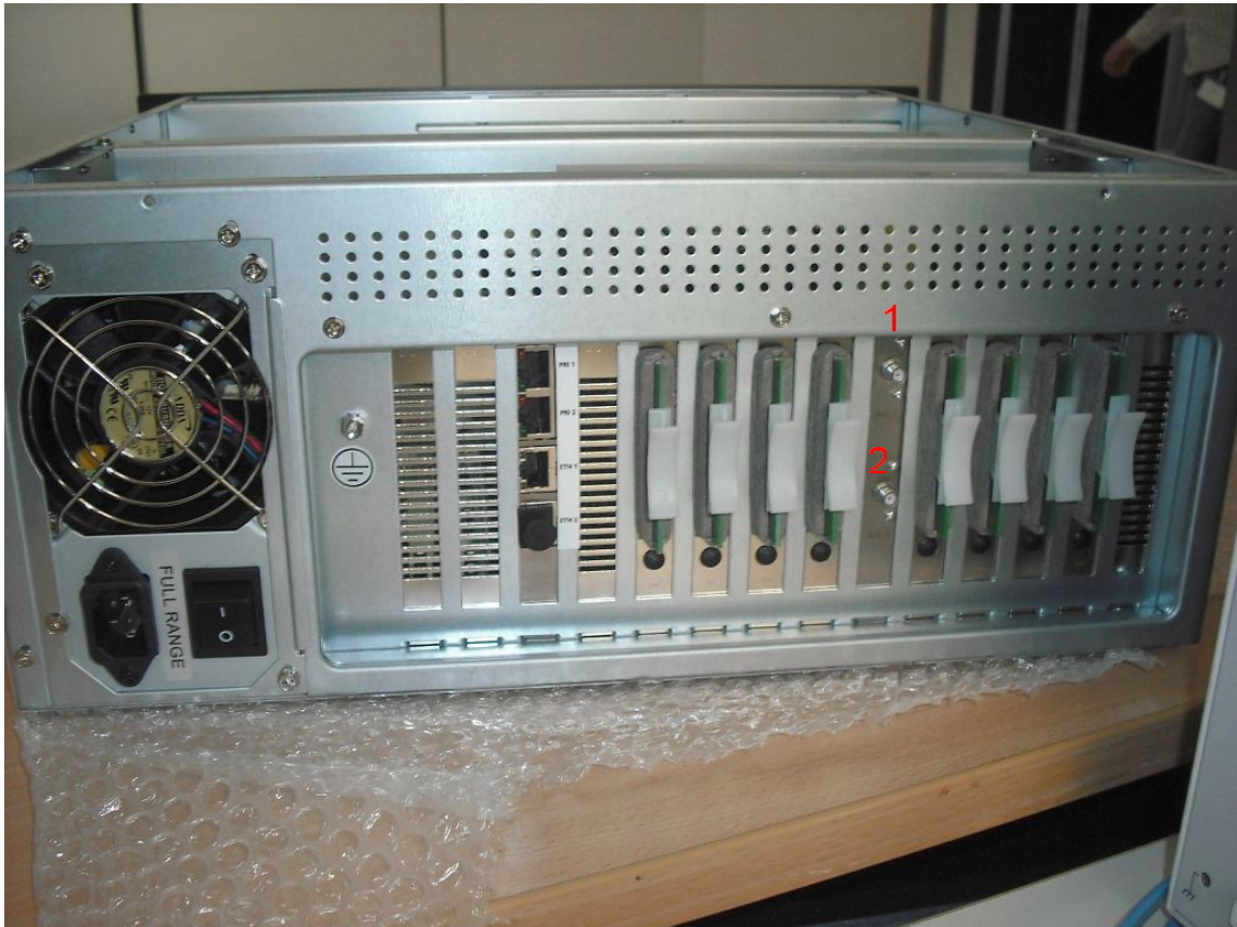
Photo 4: EUT (rear side, 8 GSM Cards inserted, 2 antenna connectors)
