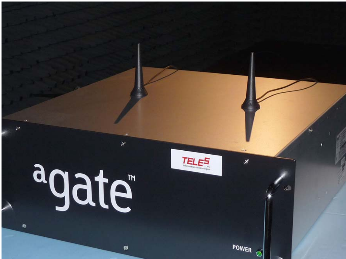
Photo 10: Assembly of both antennas on top of the housing
