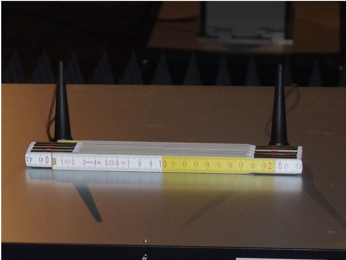
Photo 11: Distance between both antennas is 0.2 m
