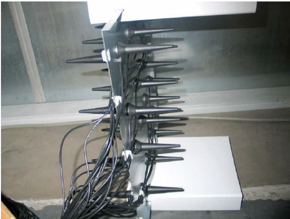
Photo 4: Assembly of antennas (16 on top side, 16 on bottom side of ground plane)
