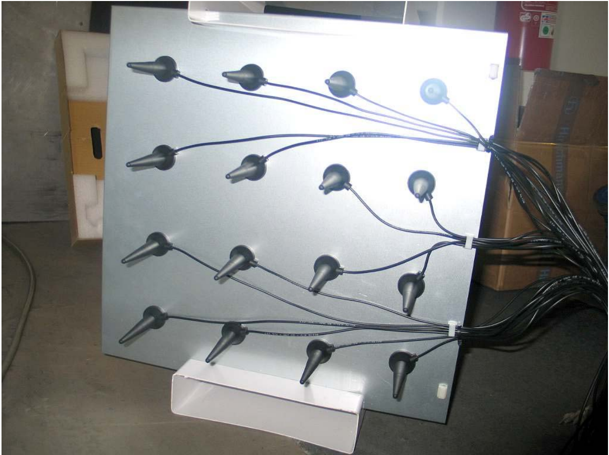
Photo 3: Assembly of antennas (shortest antenna-to-antenna distance: approx. 0.1 m)
