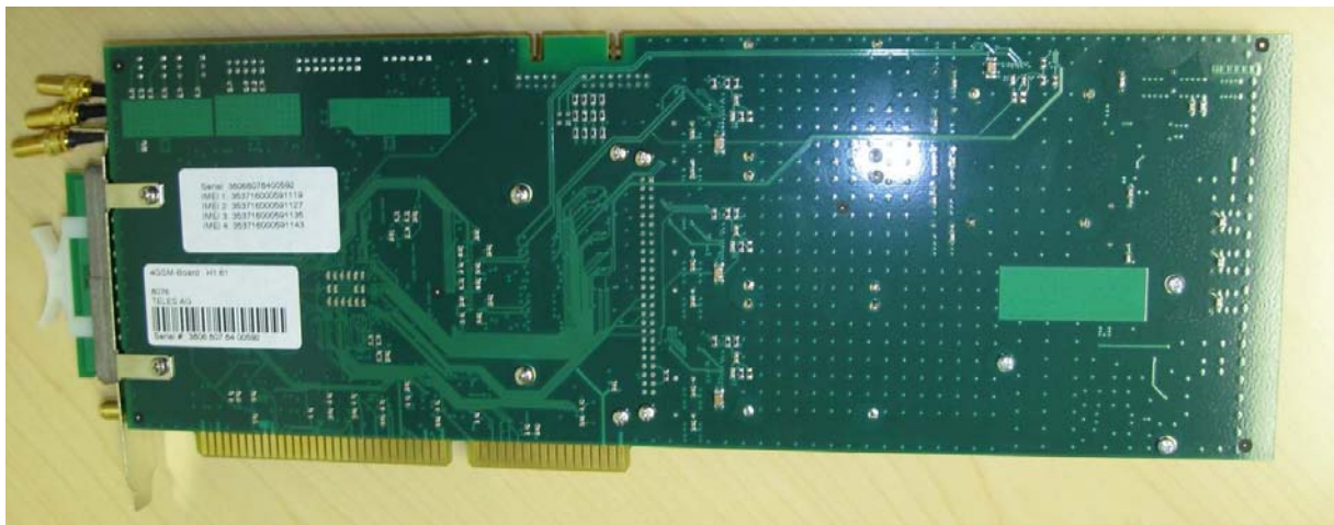
Photo 10: GSM Card, PCB (rear view)
