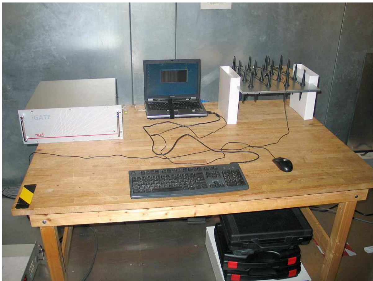
Computer peripheral set-up for conducted test
