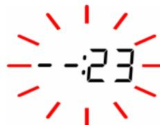
On the right side, both 7-segment character places will count the seconds. While during this, the seconds will flash during each change. The flashing separates the seconds display from the 7-segment LED on the left, which counts the minutes. A total of 60 minutes (59:59) can be shown on the display in this mode.
