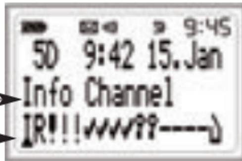
The DE920/DE940 can show a maximum of two message folders, depending on how it has been programmed. When selected the title of the message folder is displayed in the menu list. Press the confirmation key in order to display the messages in the messages folder. The messages can then be read with the help of the scroll key.
