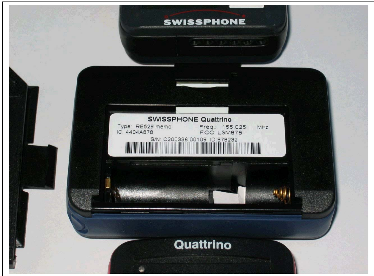
Back Side View of RE529 Model memo is shown. Diversification due to software options. Battery compartment opened for view onto label.
