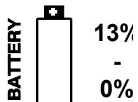
With the operation switched on, the battery symbol is permanently visible in the display, and shows the energy level at all times. If the energy source is completely used up, the empty battery symbol blinks continuously. If the acoustics are switched on, a regular beep tone is heard simultaneously. An operational time of 3 - 5 hours is still available.
