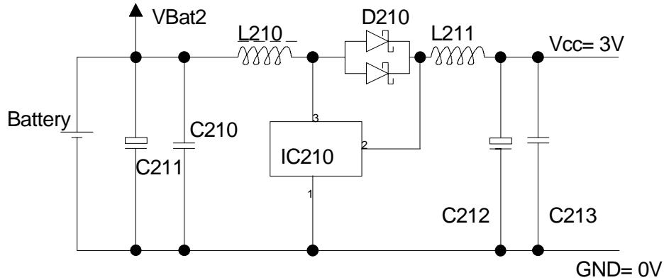
In an initial phase, the coil of IC210 is switched in for a defined period of time. The current in the coil rises. The maximum current produces the magnetic energy  $W_M = i^2 L/2$  in the coil.
