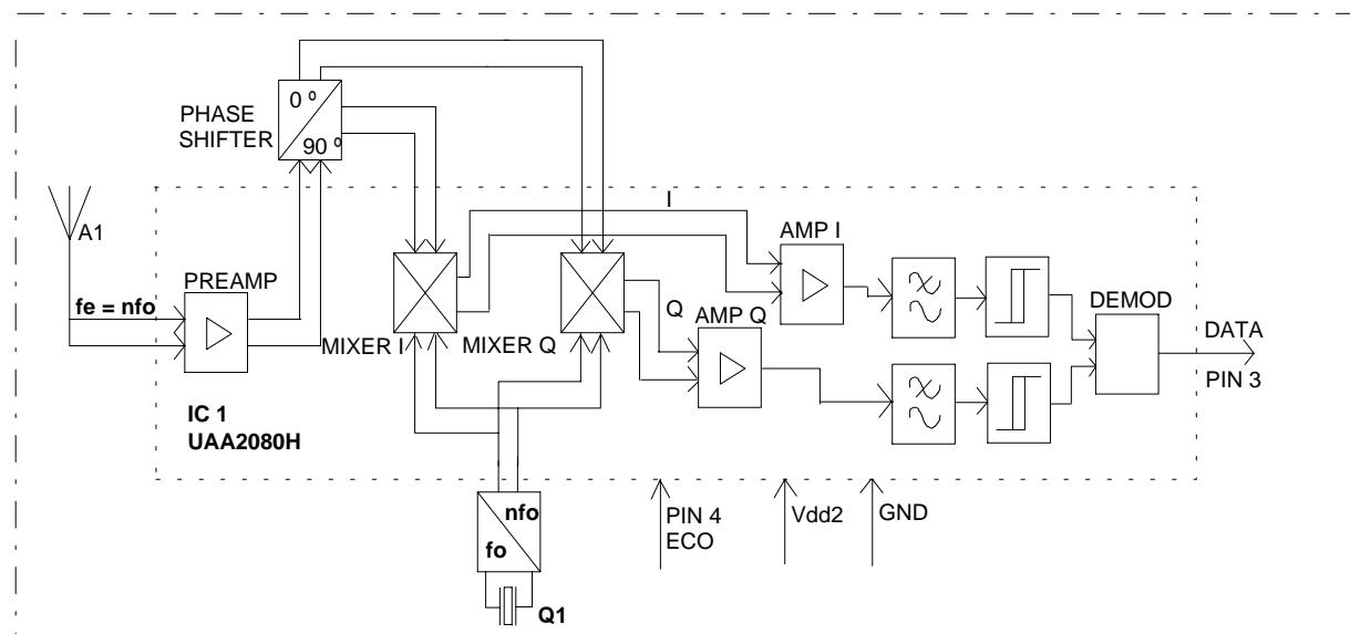
The radio signal received over antenna (A1) is amplified internally in IC1 (differential input) and is split thereafter in a phase shifter into two signals  $90^\circ$  apart from each other.
