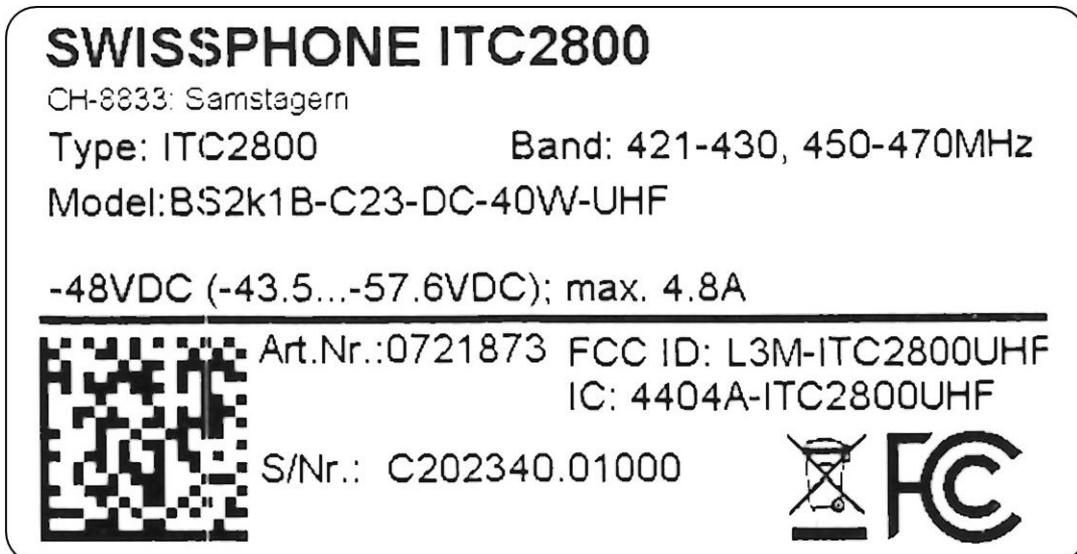
Design and parameters of the additional label for versions with the LTE module installed:
