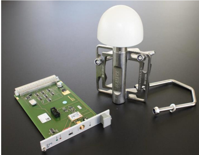
Figure 12: GPS receiver card with available GPS antenna and holder
