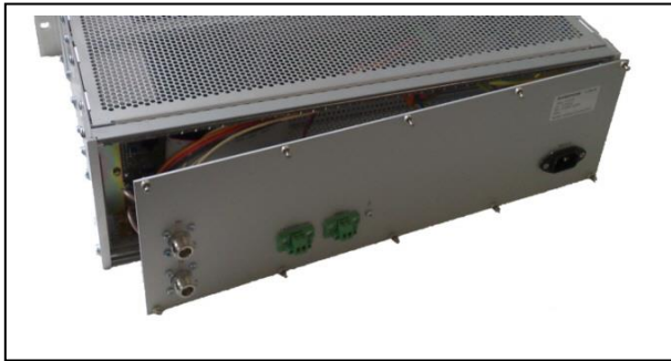
Figure 9: Removing the back panel from the ITC2500-NA
