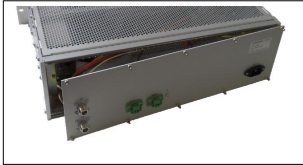
Figure 17: Removing the back panel from the ITC2500-NA
