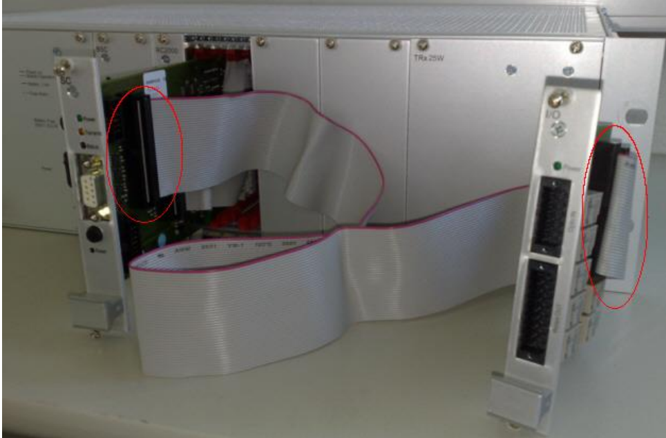
Figure 15: Connecting the I/O card to the ITC2500-NA
