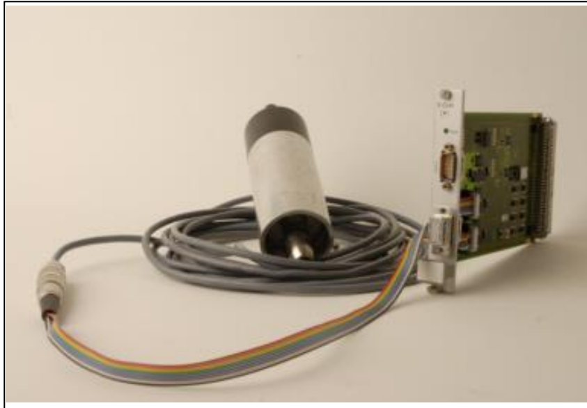
Fig. 7-9: GPS interface card (S-Com) and GPS antenna
