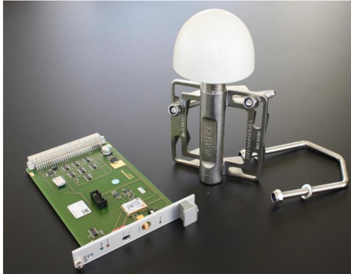
Fig. 5-8: GPS receiver card with potential GPS antenna and fixture
