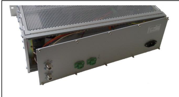
Fig. 5-4: Removing the ITC2100-NA back panel
