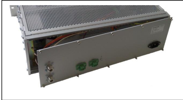
Fig. 5-13: Removing the ITC2100-NA rear panel
