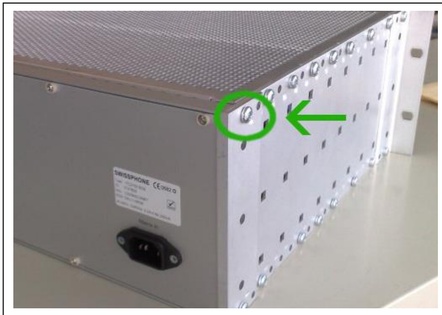
Fig. 5-1: Grounding point at ITC2100-NA
