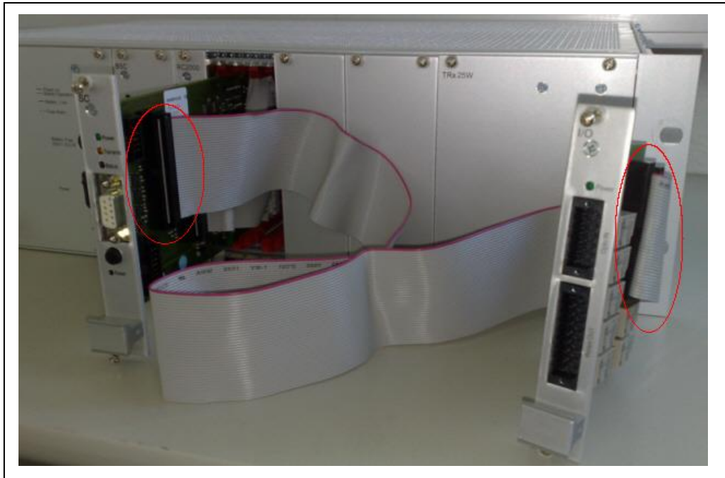
Fig. 5-11: Connection of the I/O to the ITC2100-NA
