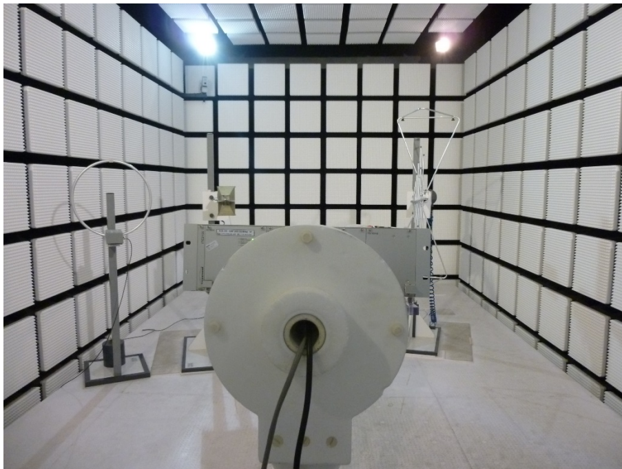
Photo 3: Measurements fully anechoic chamber
