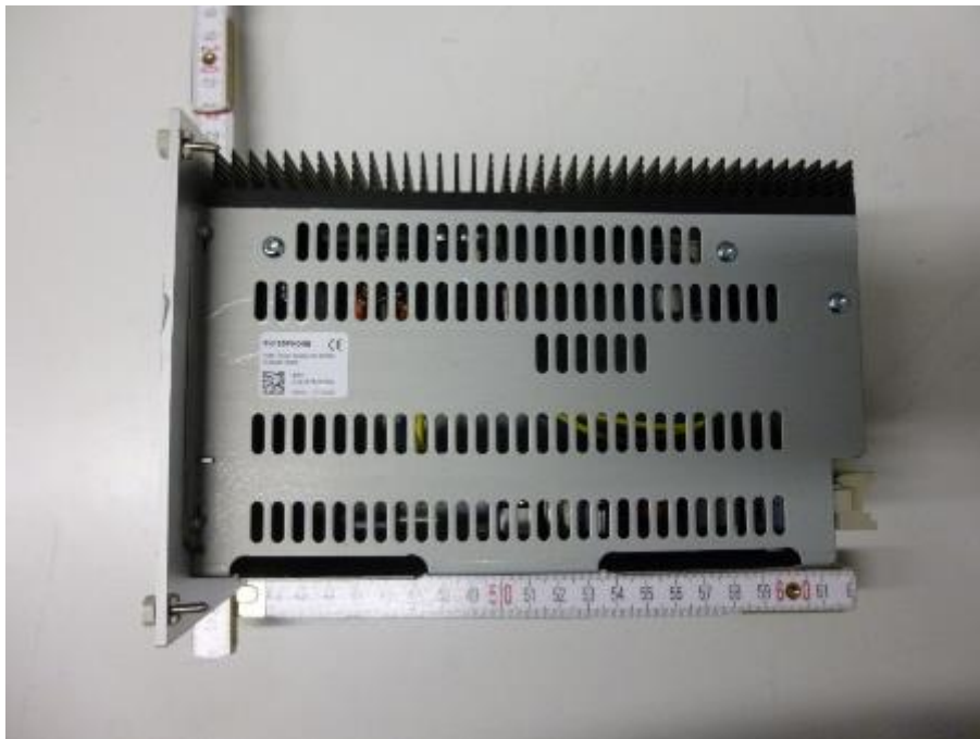
Photo 5: Power supply module
