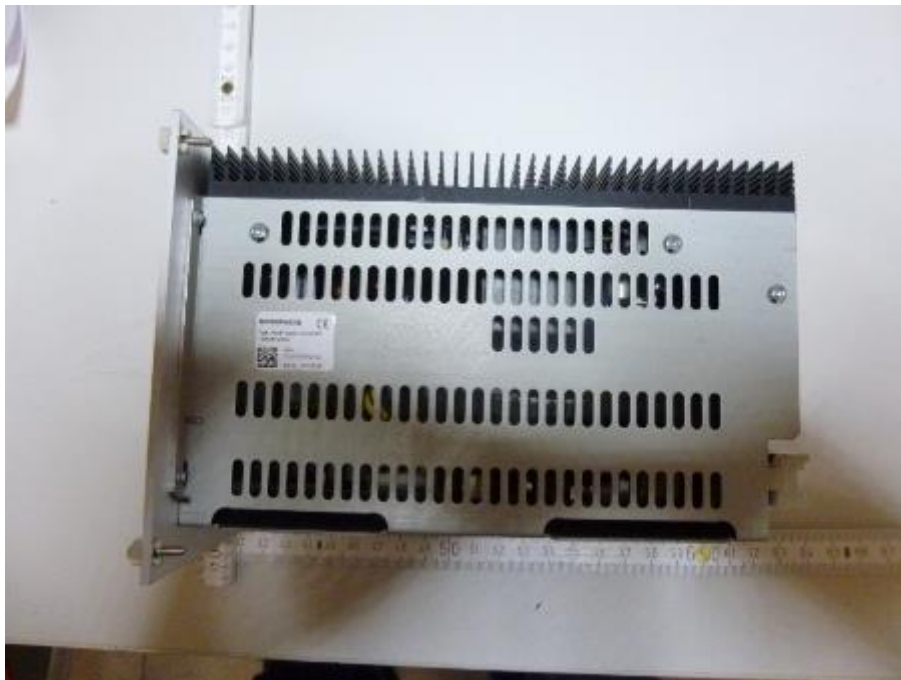
Photo 5: Power supply module
