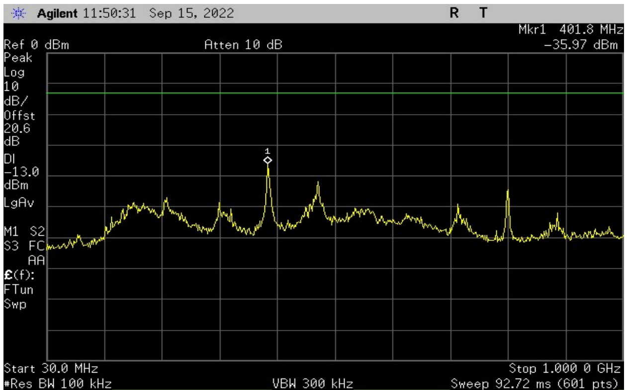
Plot 8 – Lowest Channel - 30MHz to 1GHz
