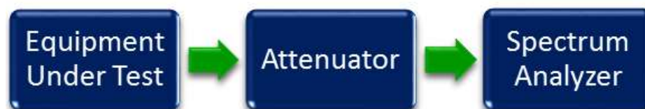
Figure 3: Spurious Emission at Antenna Terminal Test setup
