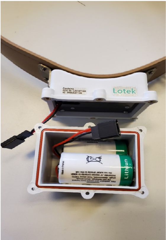
Housing Opened Up Front View – Internal Antenna
