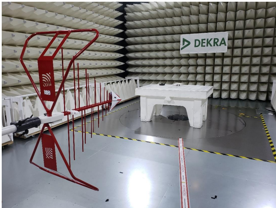
6. Low Range Radiated Emission test setup (30MHz to 1GHz)
