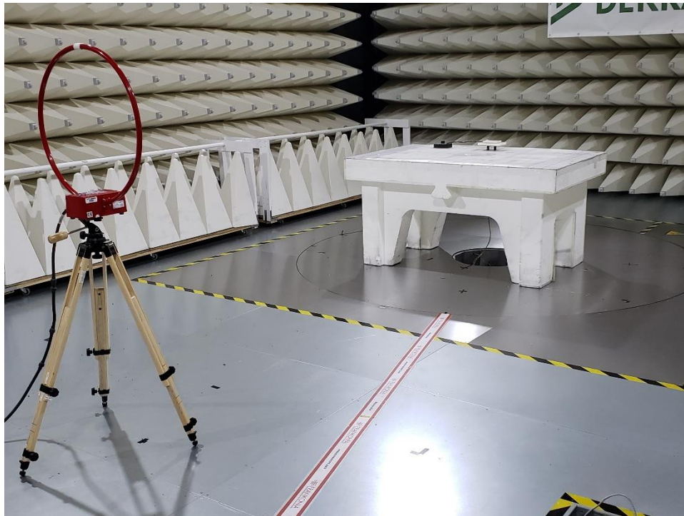
7. Low Range Radiated Emission test setup 9KHz to 30MHz
