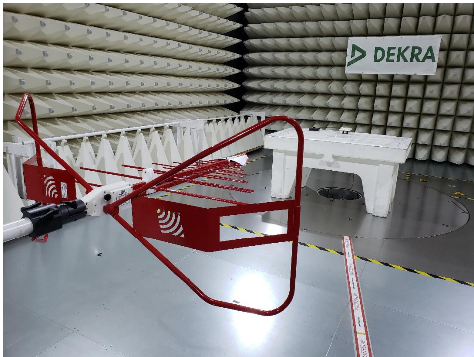
8. Low Range Radiated Emission test setup (30MHz to 1GHz)
