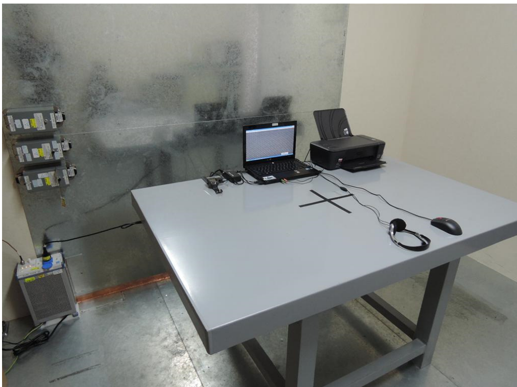
Photograph 6: Set-up for for Mains Conducted testing Front
