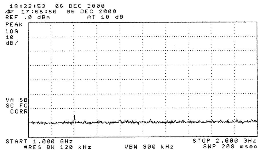
Figure 5.2. Emissions measured at 3 meters in anechoic chamber, 1000-2000 MHz.
