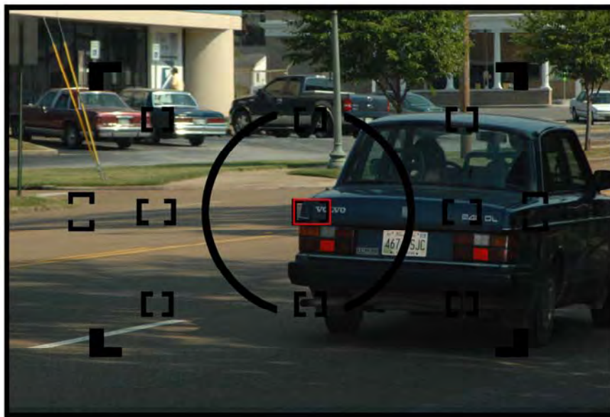
Vehicle in Near Lane When Furthest Lane Was Focused
