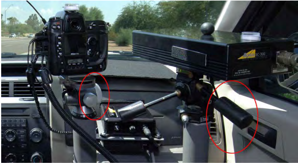
Vertical Adjustment Tripod Handle and Tripod Mount Knobs
