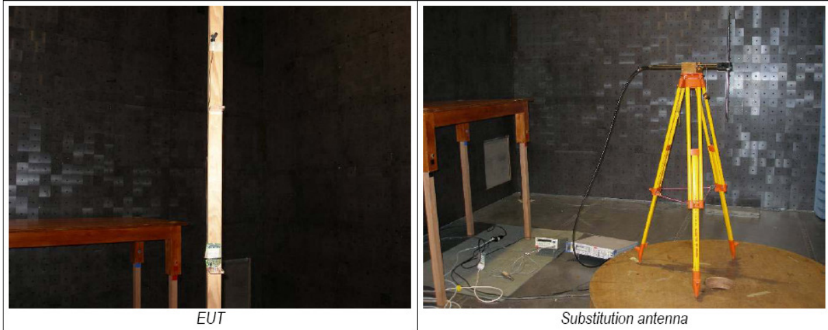
Fig 1 RF Power output measurements
