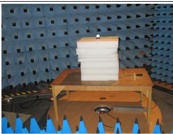
Fig 2 Radiated measurements – carrier and band edge
