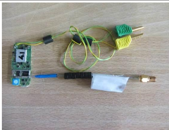
Electronic board with temporary antenna &amp; supply connectors
