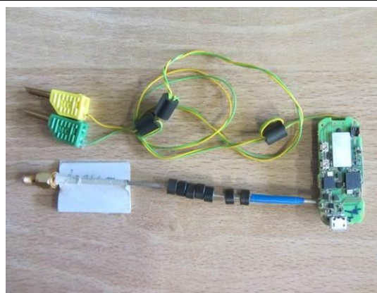
Electronic board with temporary antenna &amp; supply connectors
