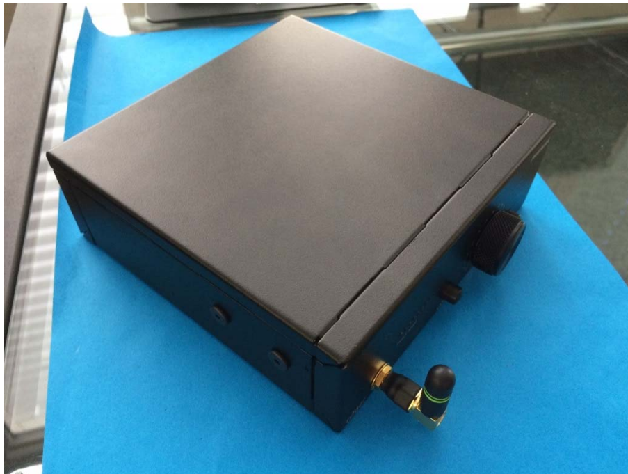
Photo 7: End product with permanently fixed antenna
