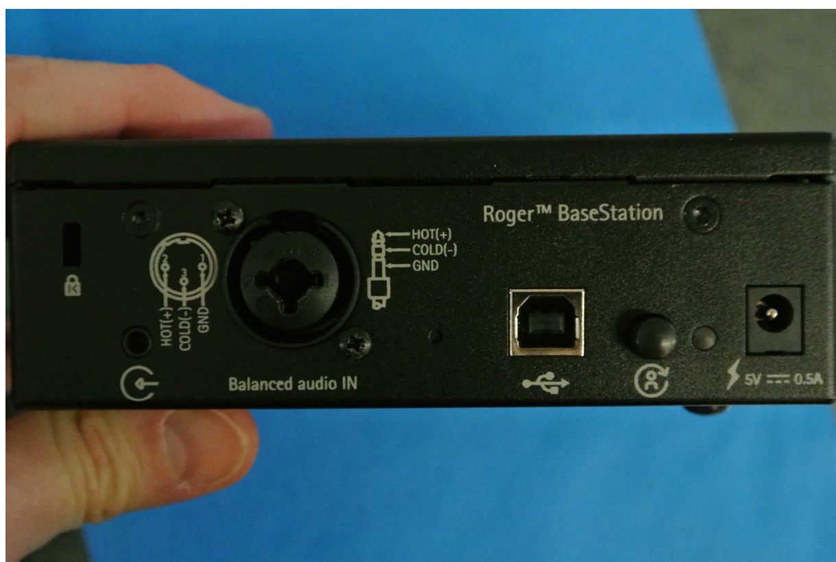
Figure 3: Marking on the backplate of Roger BaseStation
