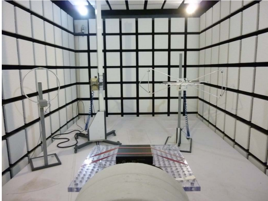
Photo 3: Anechoic chamber test setup
