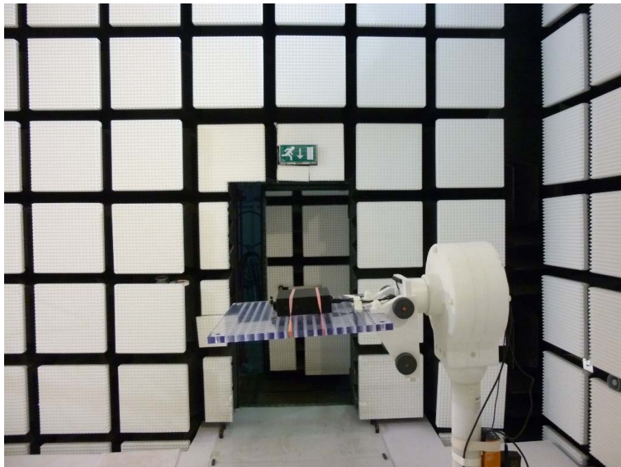
Photo 4: Anechoic chamber test setup
