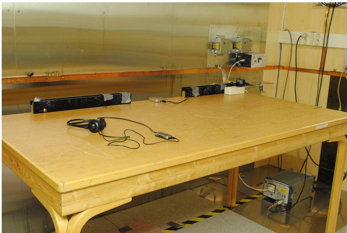
Power line Conducted Emissions
