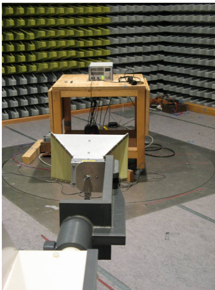
Figure 6-4: Test setup for radiated emission measurement, 1 GHz to 15 GHz
