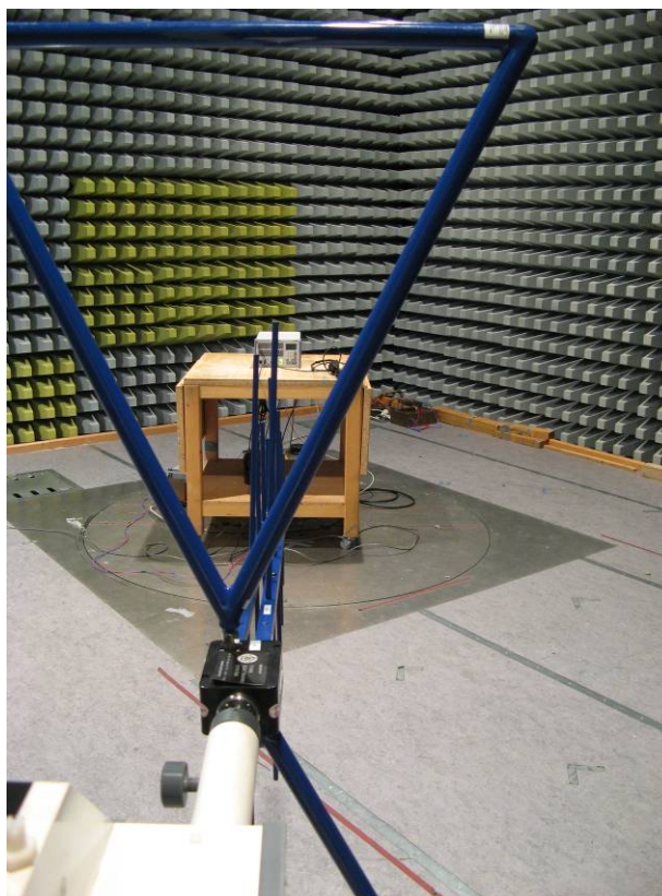
Figure 6-1: Test setup for radiated emission measurement, 30
