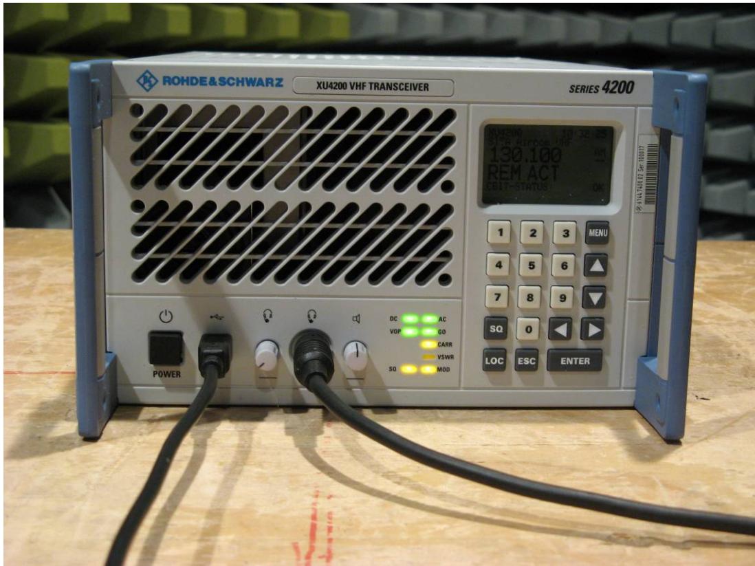
Figure 4-1: XU4200 VHF Transceiver (EUT), front view
