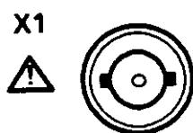
With Transceiver XU 221, the recessed BNC socket X1 is intended for the connection of an external synthesizer. For this purpose, the internal RF cable must be pulled off connector X94 of the internal synthesizer and be re-connected to X1.
