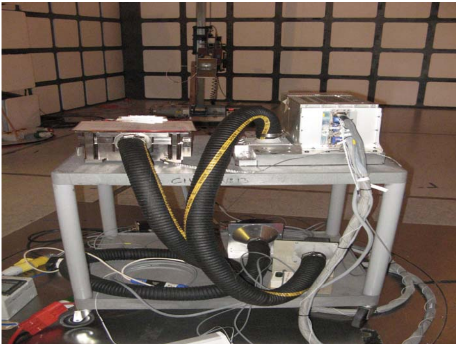
Radiated Emissions – 1GHz to 18GHz
