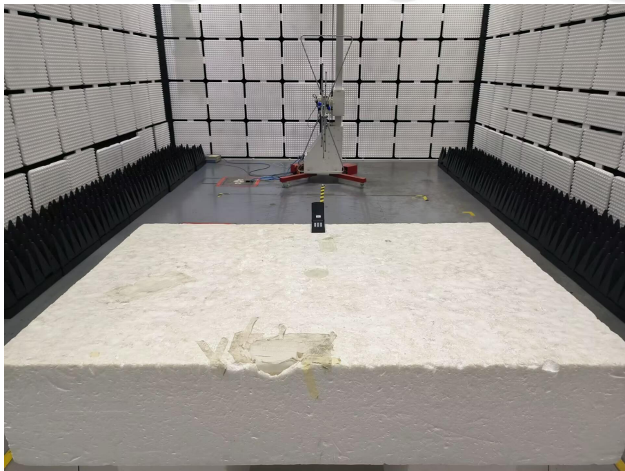
Radiated emission Test Setup-1 (30MHz ~ 1GHz)
