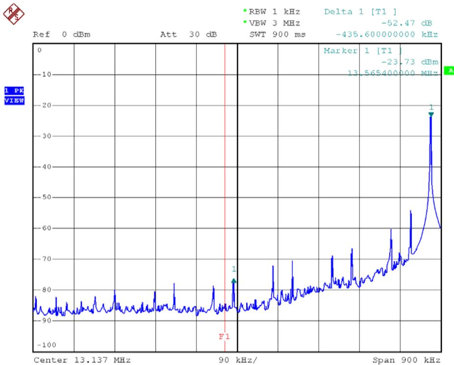
Bandwidth / Bandedge Plot – Pursuant to FCC Part 15 Section 15. 225 Requirement
