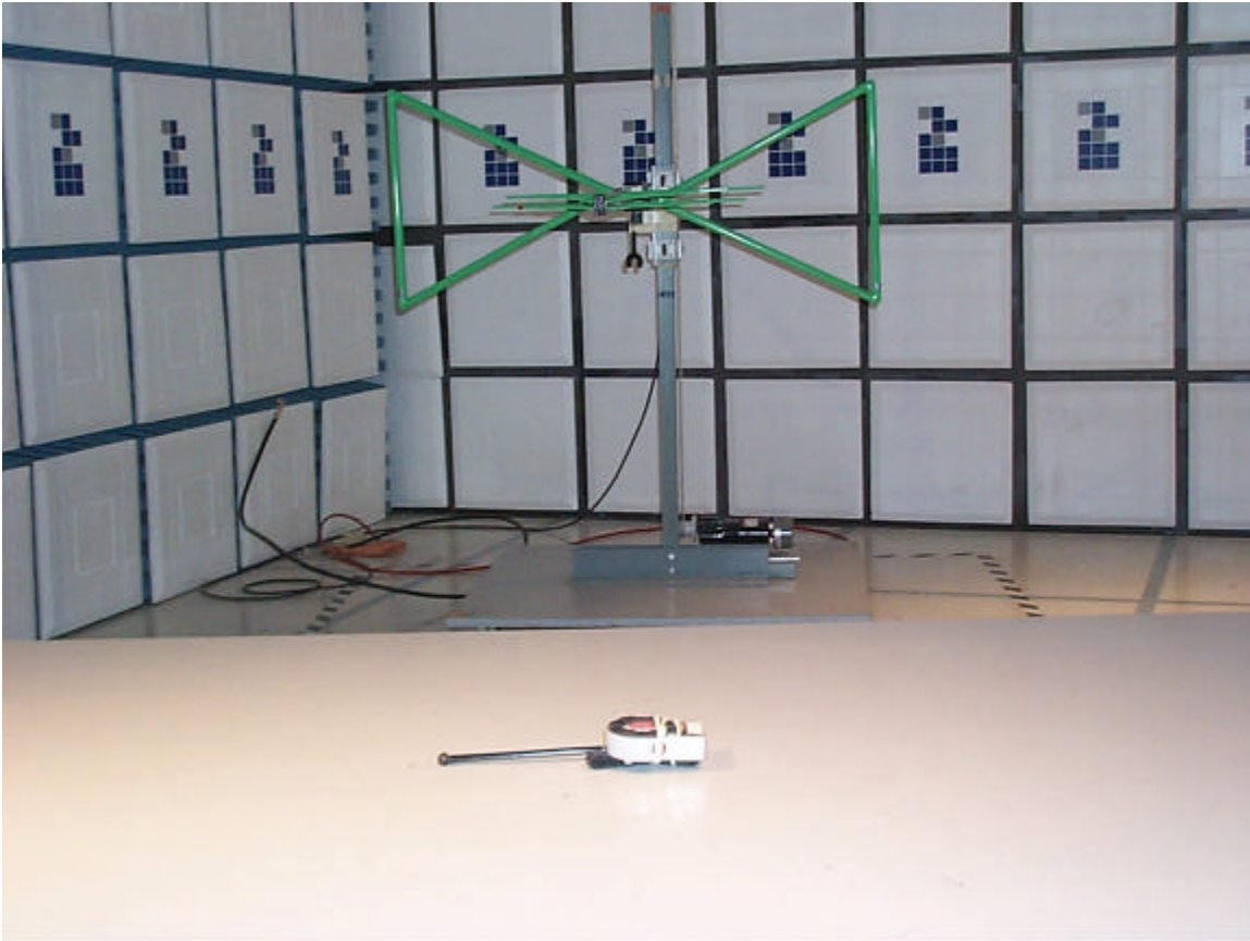
Maximized Radiated Emission Test Set-up Horizontal Polarization
