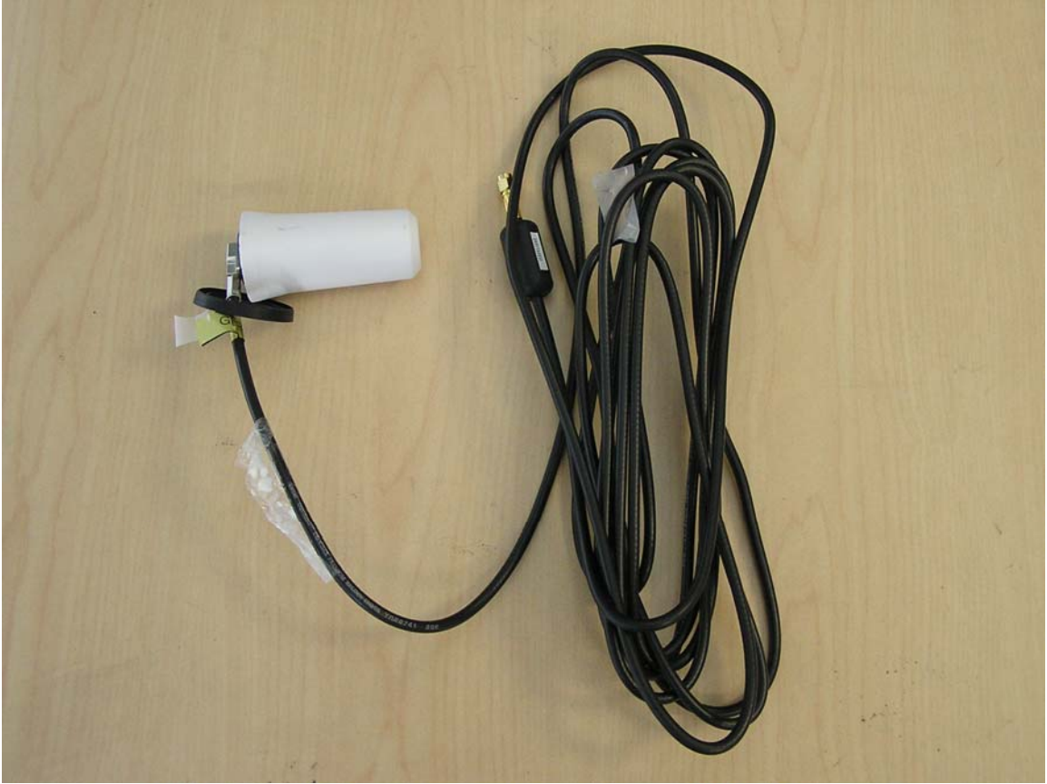
Dual band roof type Patch antenna
