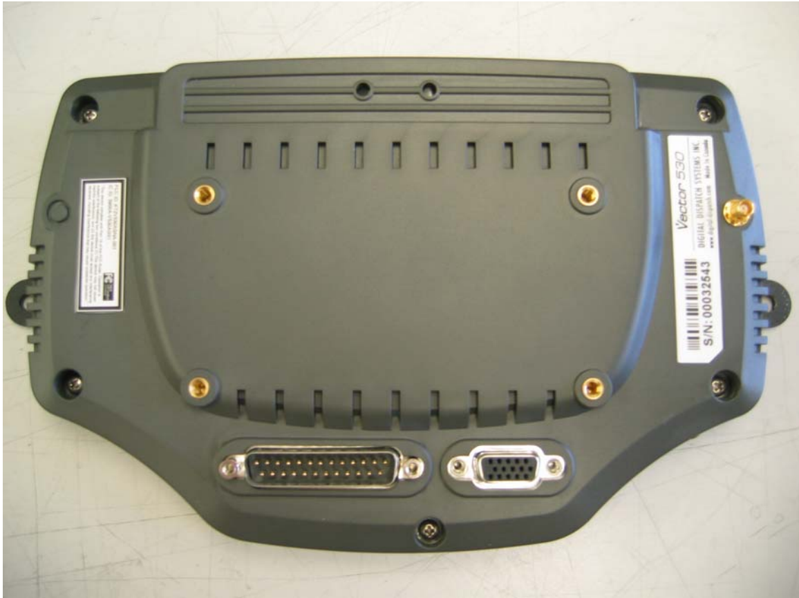
EUT model# Vector 530 AVL GPRS-NA – Bottom view
