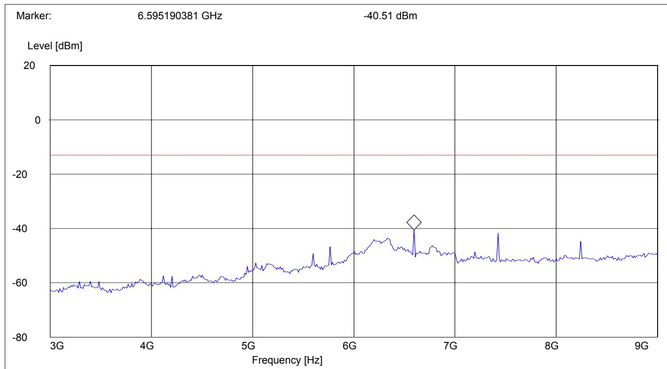
**RADIATED SPURIOUS EMISSIONS (GSM-850)****Tx @ 836.6MHz: 1GHz – 1.58GHz**
