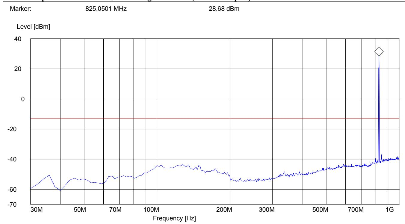
**RADIATED SPURIOUS EMISSIONS (GSM-850)****30MHz - 1GHz**
