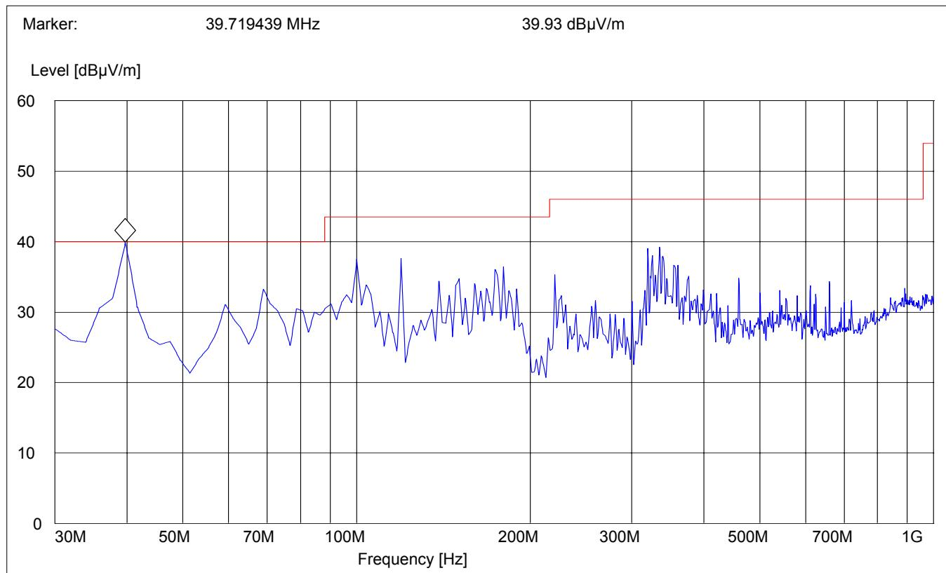
**RECEIVER RADIATED EMISSIONS****EUT in Idle Mode: 30MHz – 1GHz****Antenna: horizontal****SWEEP TABLE: "FCC Spur 30M-1G"**
