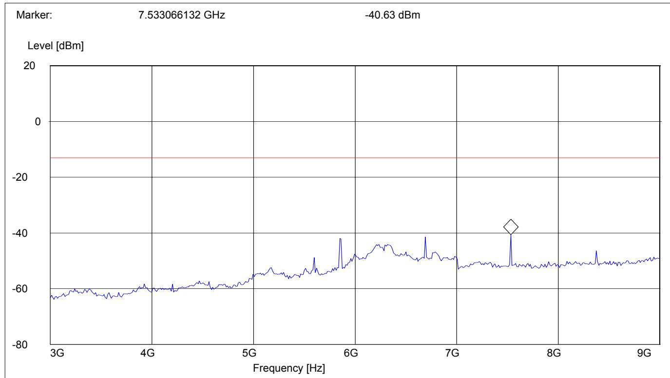
**RADIATED SPURIOUS EMISSIONS (GSM-850)****Tx @ 848.8MHz: 1GHz – 1.58GHz**
