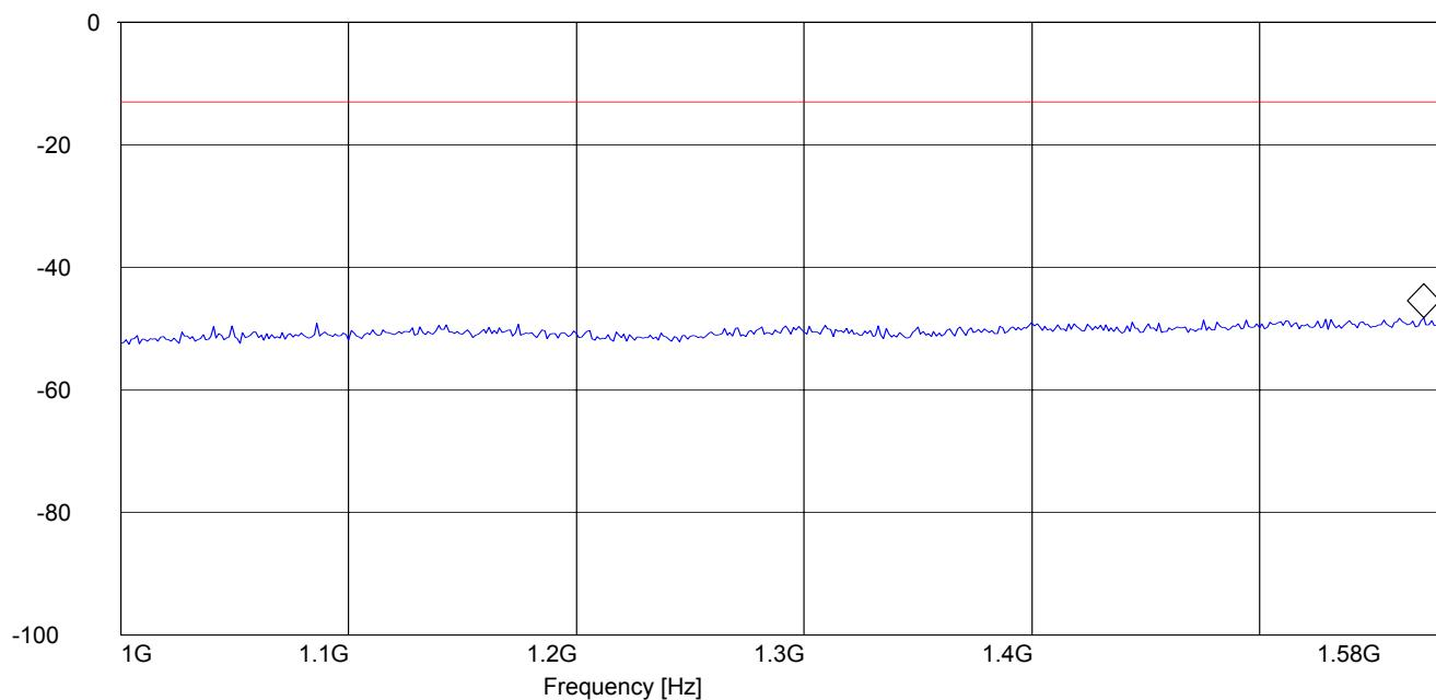
**RADIATED SPURIOUS EMISSIONS (GSM-850)****Tx @ 848.8MHz: 1.58GHz – 3GHz**
