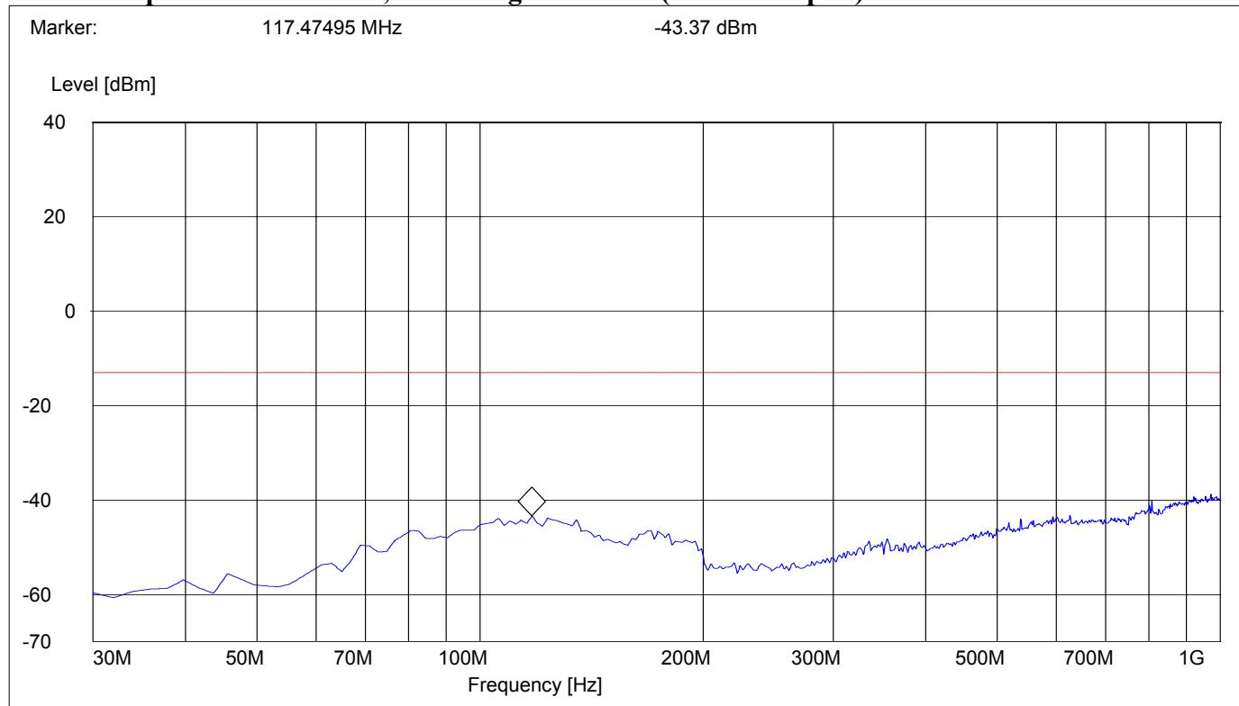
**RADIATED SPURIOUS EMISSIONS****30MHz - 1GHz**
