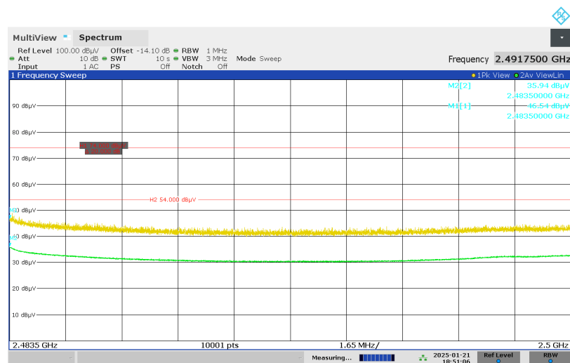
Figure 36: Restricted-band Band-edge, Spectral Diagram, Horizontal Antenna Orientation, BLE, Mode H (2480MHz), 2Mbps
