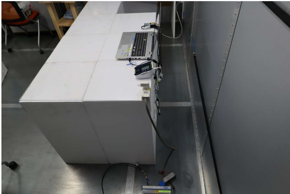
Photograph 9: Set-up for AC Power Line Conducted Emission, Rear View
