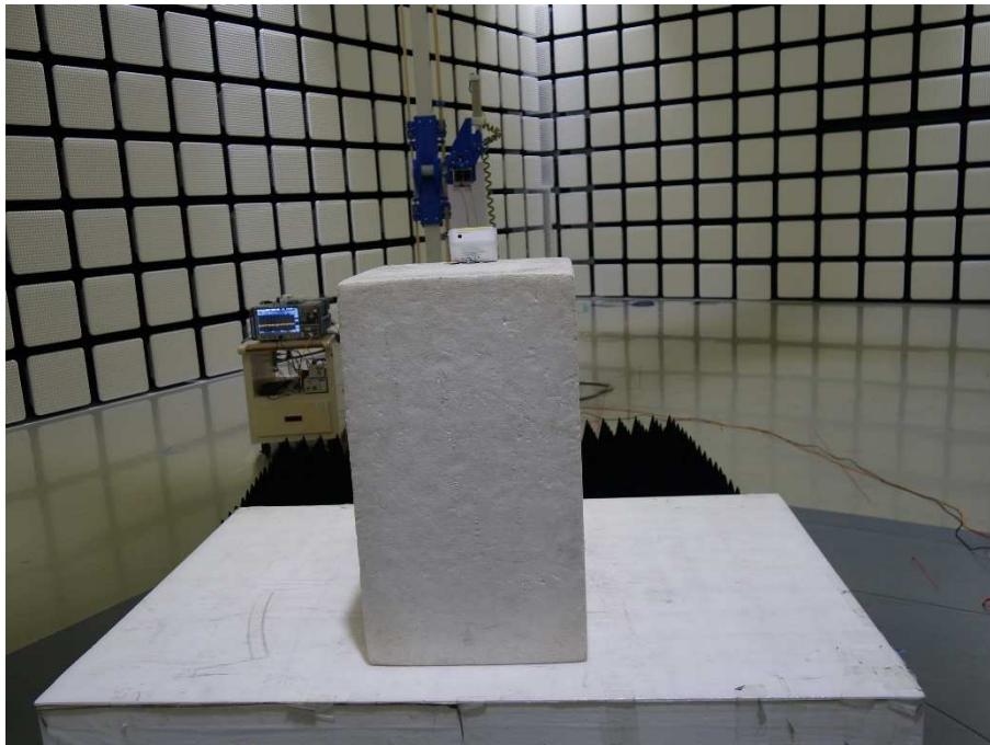
Photograph 7: Set-up for Radiated Spurious Emission above 1GHz, Rear View
