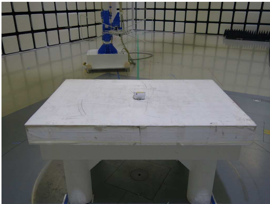
Photograph 5: Set-up for Radiated Spurious Emission below 1GHz, Rear View
