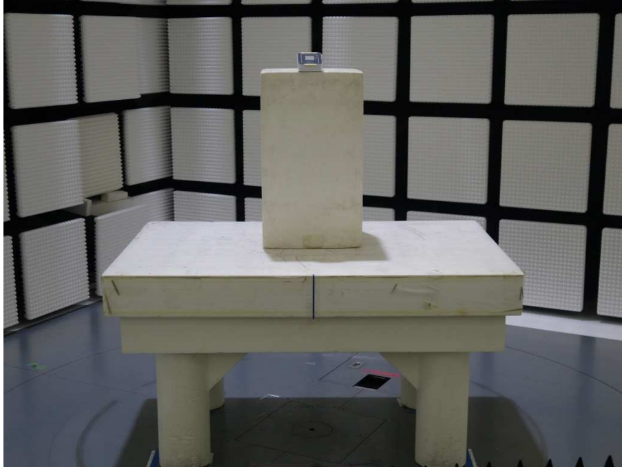
Photograph 6: Set-up for Radiated Spurious Emission above 1GHz, Front View
