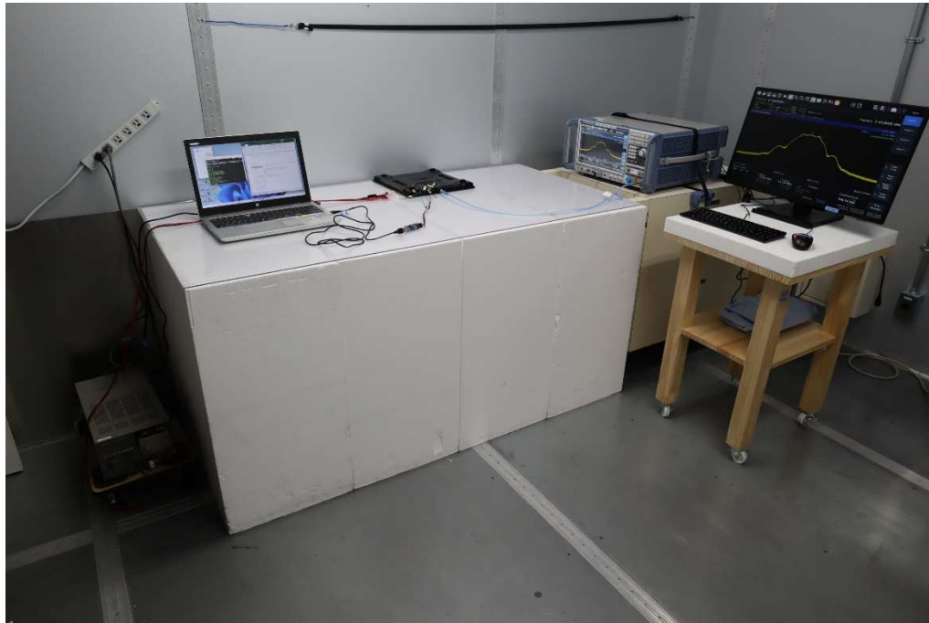
Photograph 1: Set-up for Antenna Port Conducted Emission of Transmitter, General View
