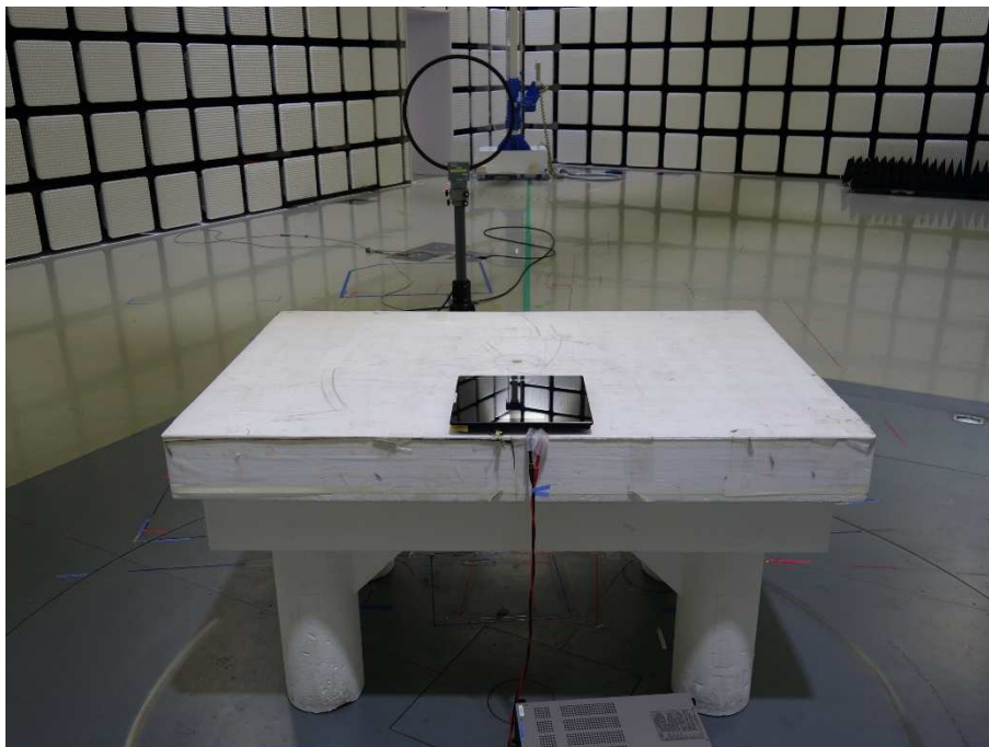
Photograph 3: Set-up for Radiated Spurious Emission below 30MHz, Rear View
