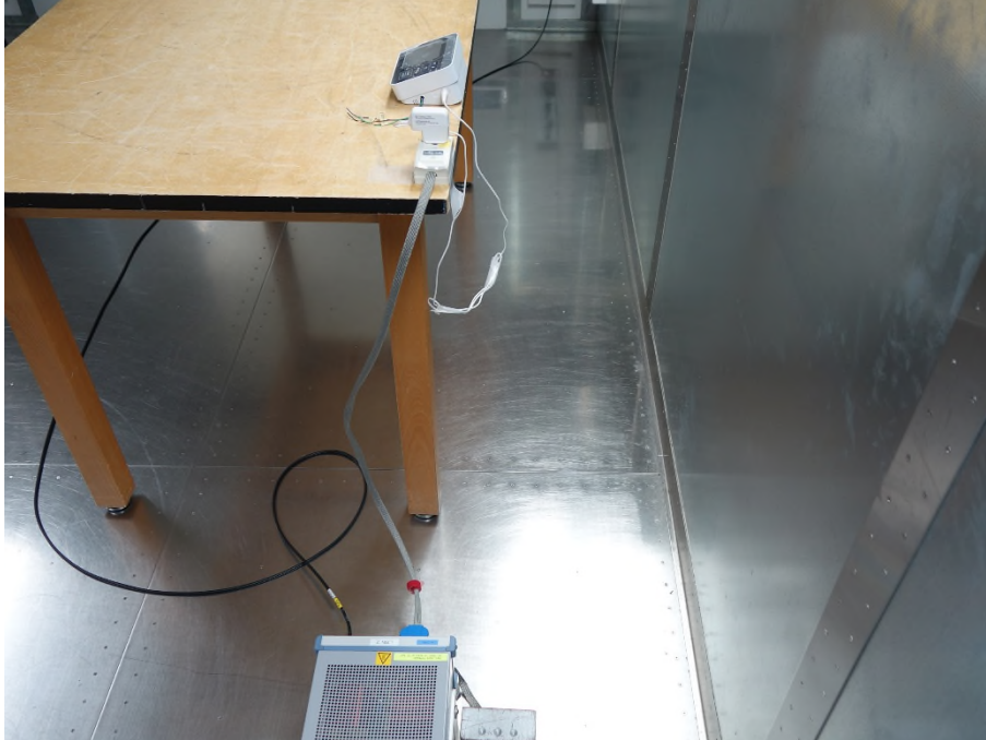
Photograph 9: Set-up for AC Power Line Conducted Emission, Rear View
