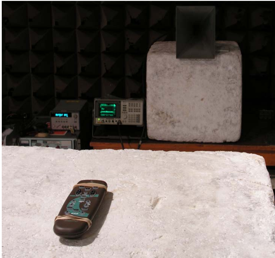
Test Setup (Radiated Emissions) – one of three axes tested
