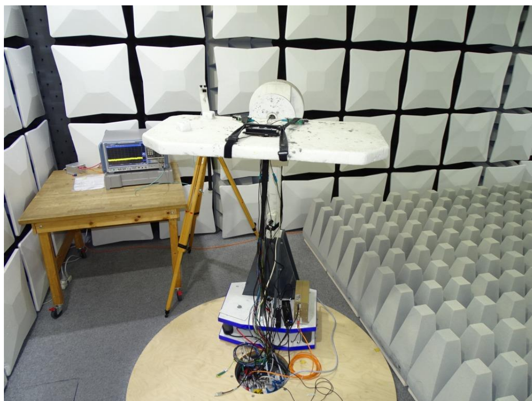
Photo 4: Test setup for radiated measurements above 26 GHz
