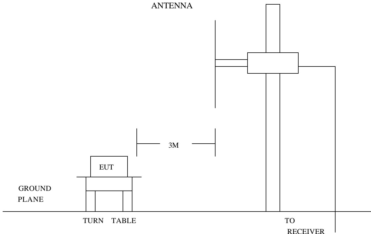
**5 . 3 RADIATED TEST SET-UP**
