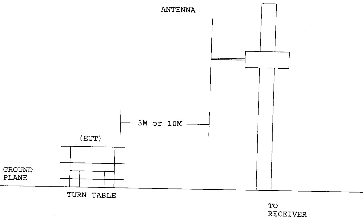
6.5 RADIATED TEST SETUP
