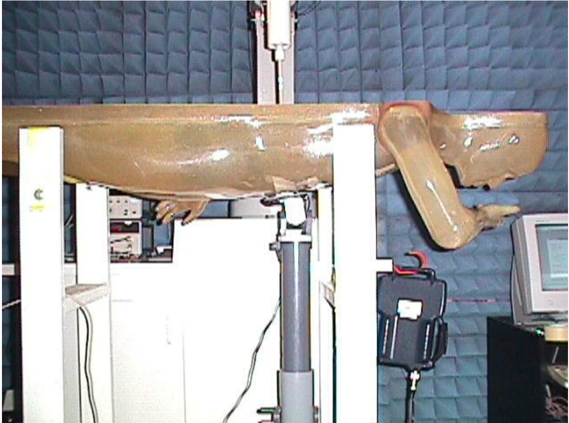
< Waist with the Aerocomm, NZH2400-MMCX microstrip antenna, 10mW unit - Overview >
