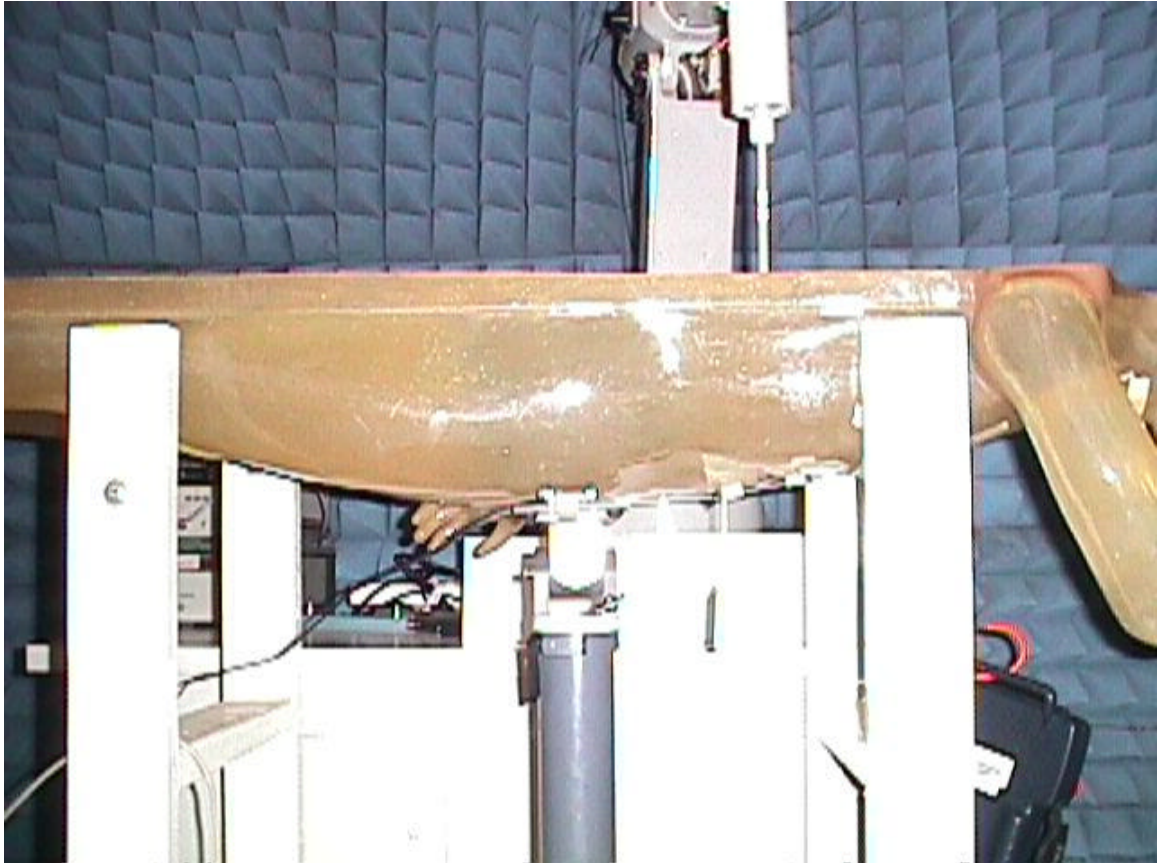
< Waist with the Nearson, S131CL-5-RMM-2450S ¼ wave dipole antenna, 10mW unit – Overview >
