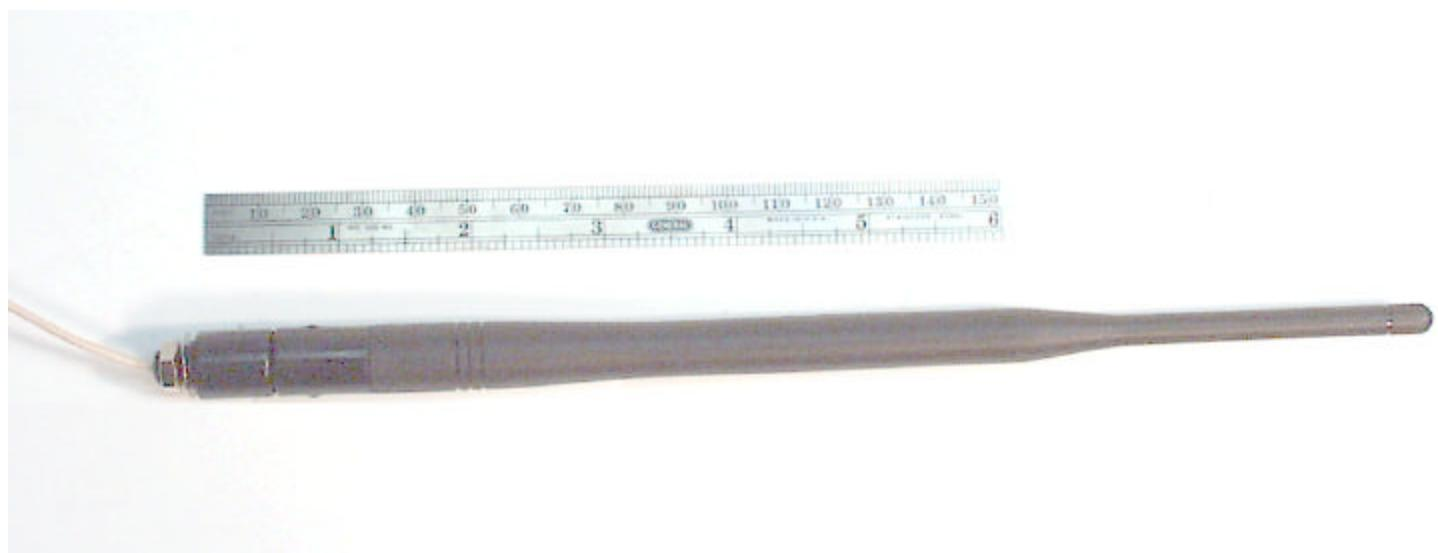
**Nearson S191FL-5-RMM-2450S 3/4 Wave Dipole Antenna**
