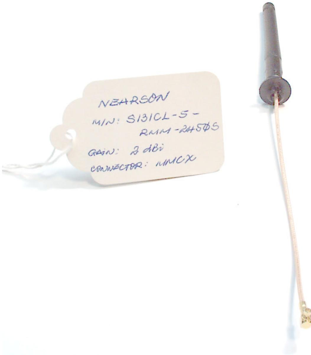
**Nearson S181FL-5-RMM-2450S 1/4 Wave Dipole Antenna**
