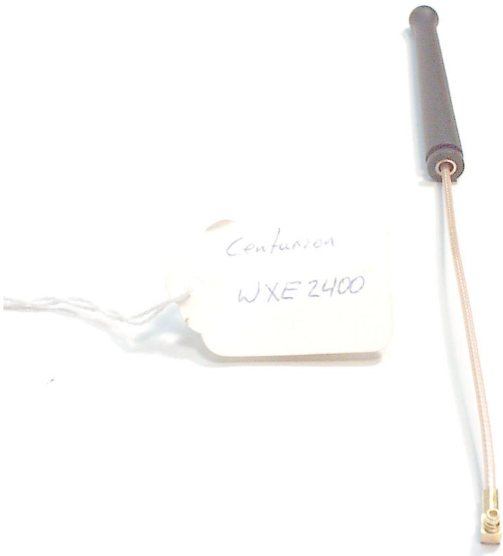
**Nearson S131CL-5-RMM-2450S 1/4 Wave Dipole Antenna**
