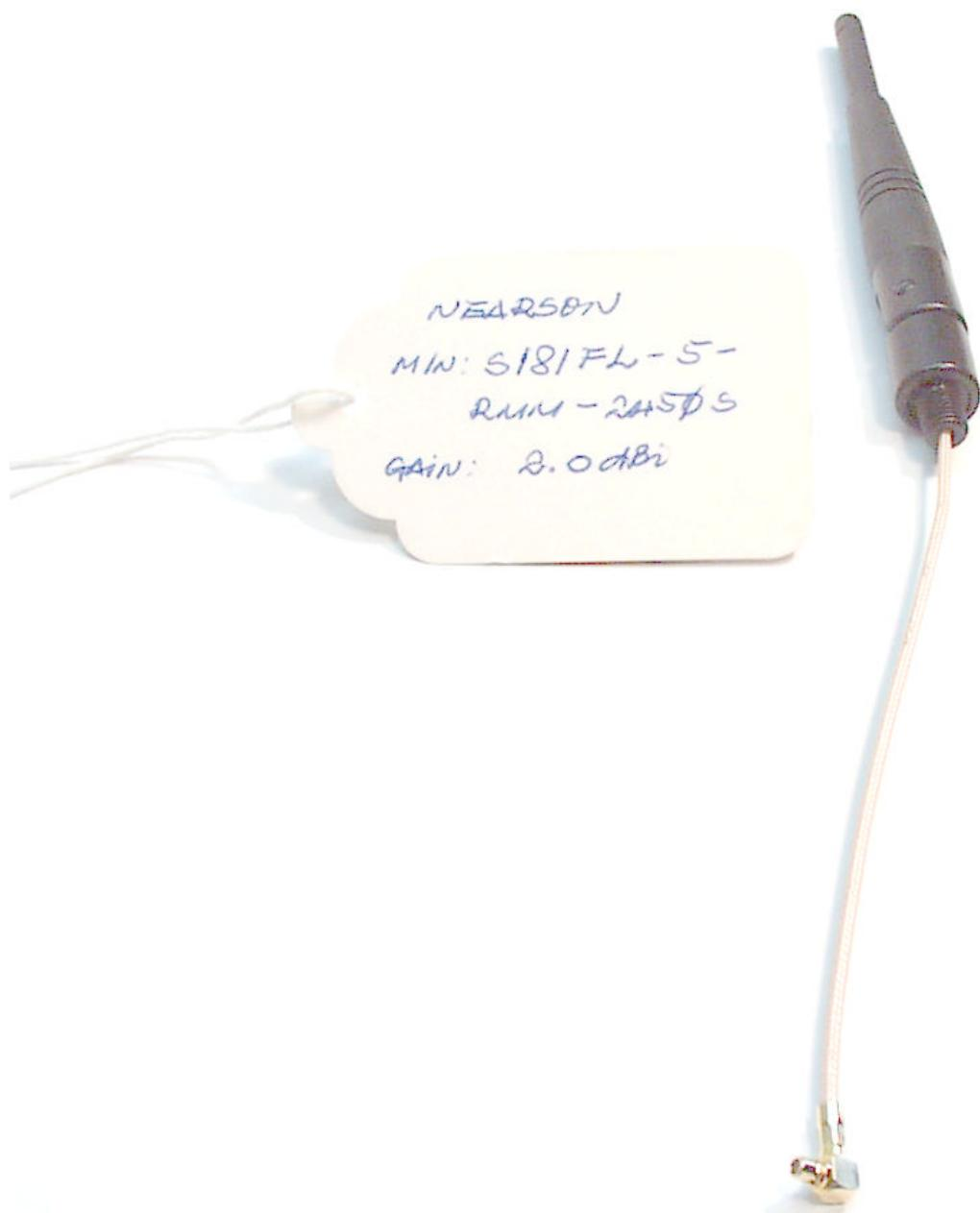
**Nearson S191FL-5-RMM-2450S 3/4 Wave Dipole Antenna**
