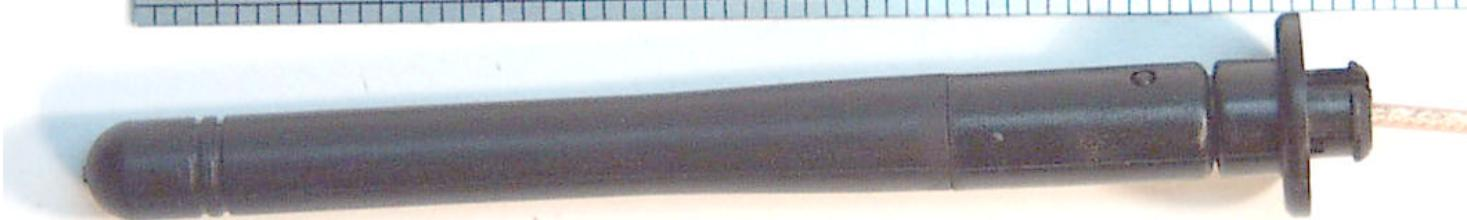
**Nearson S131CL-5-RMM-2450S 1/4 Wave Dipole Antenna**
