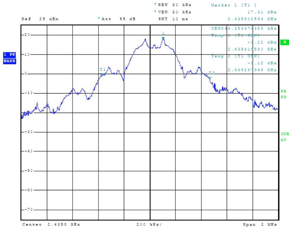
Figure Seventeen Plot of 20 dB Occupied Bandwidth (79 Hop Set)
